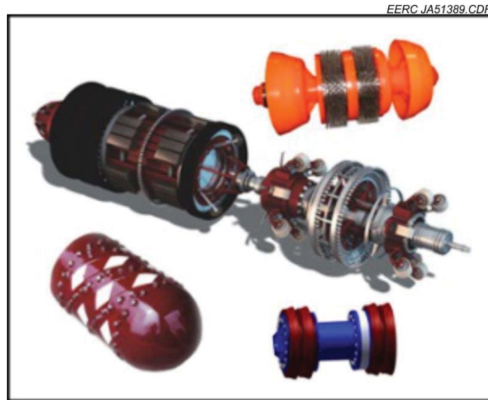
Figure 43. Illustration of pig types.
