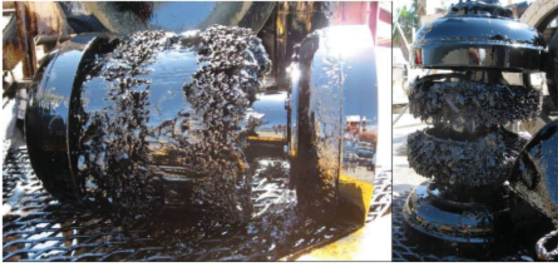
Figure 45. Brush pig after emerging from Cleaning Run 2.
