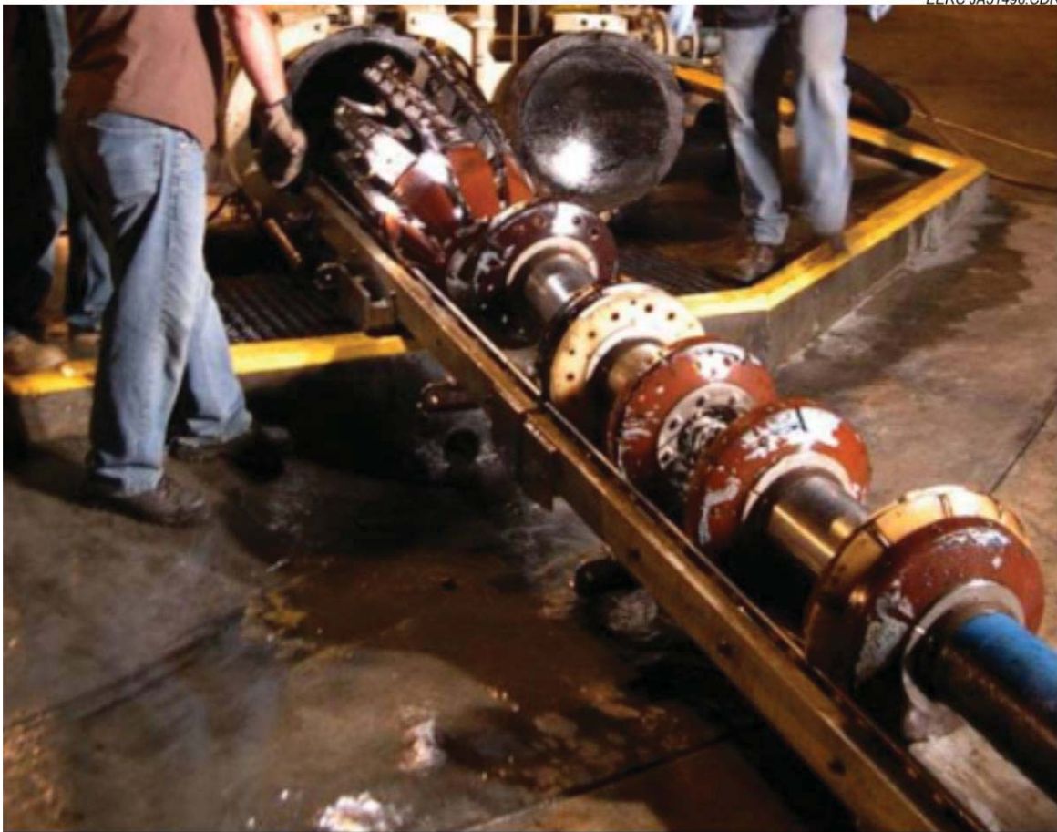
Figure 46. Intelligent pig after integrity determination run following three-stage chemically assisted pigging operation—note cleanliness.
