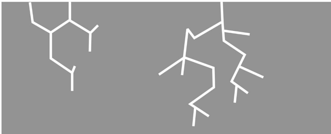
Figure E-5. Different crack shapes depending on the type of SCC.
