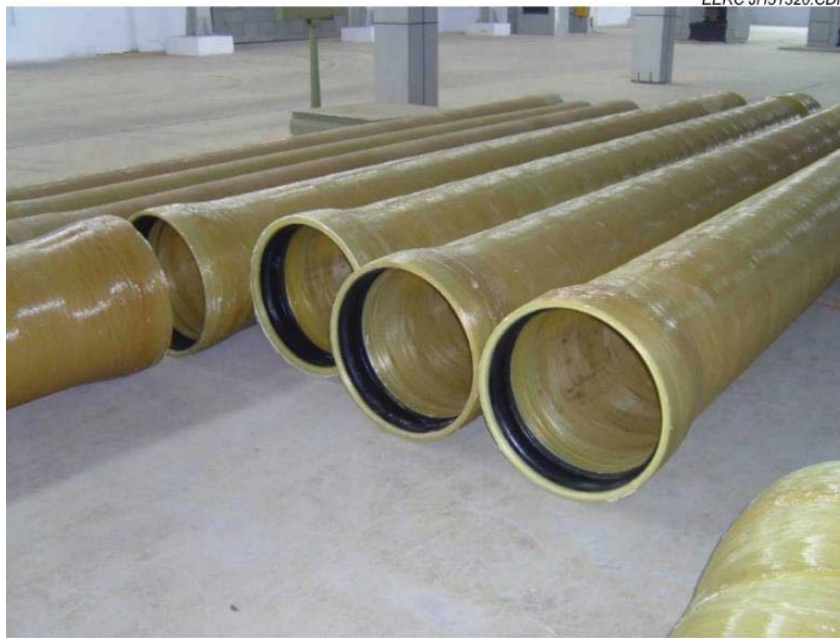
Figure 31. Fiberglass pipeline segments.
